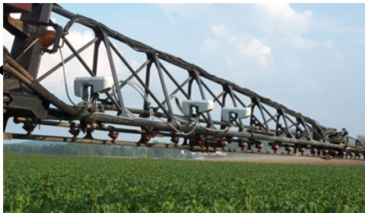
Sensors mounted on the spray boom of a hi-boy sprayer take NDVI readings based on the biomass, or leaf density, of the cotton plants.
